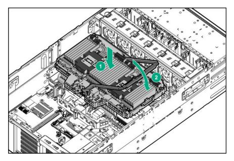
11. Install the air baffle (Installing the air baffle on page 41).
