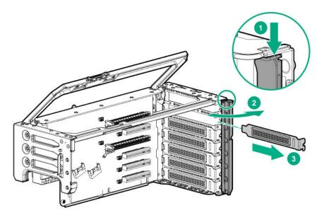
8. Install the controller into the PCI riser cage.
