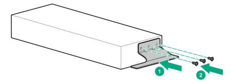
Install the GPU card into the riser cage.
