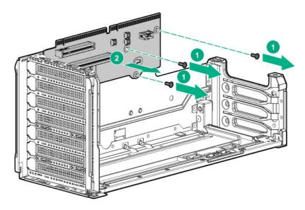
**9.** Align the screw holes on the riser board with the holes on the riser cage, and then install the riser board.
