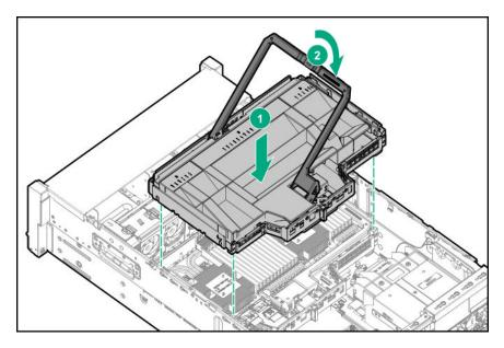
10. Install the air baffle (Installing the air baffle on page 41).
