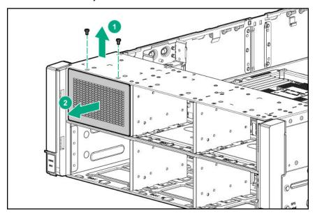
12. If installed in the server, remove the universal media bay.
