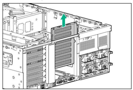
**b.** Remove the tertiary slot blank.
