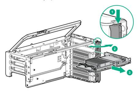
8. Remove the riser board installed in the riser cage.
