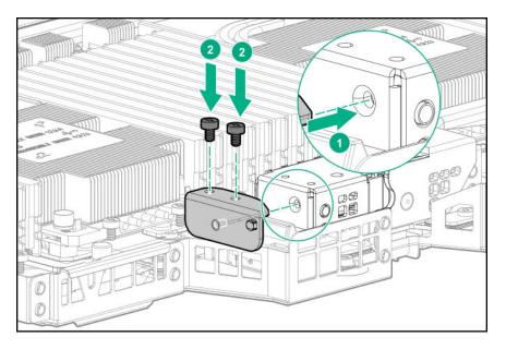
**12.** Install the mezzanine card. Listen for a click to indicate that the card is fully installed when the handle is closed.
