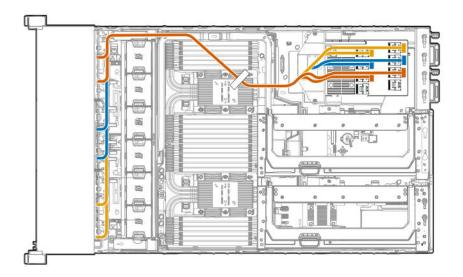
b. Route the cables from the lower drive box backplanes (boxes 4-6) to the SAS expander card in the primary riser cage.
