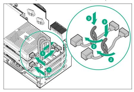
Tuck the looped cables between the GPU cards and the riser cage.
