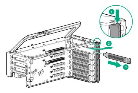
7. Install the expansion board into the PCI riser cage.
